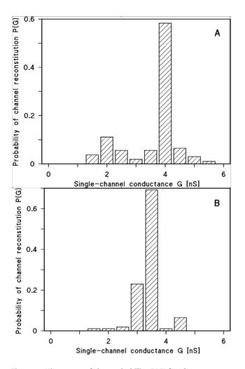
Figure 3. Histogram of the probability P(G) for the occurrence of a given conductivity unit. Probability observed with lipid bilayer membranes in the presence of OmpF alone (A) or when the aqueous phase contained in addition 0.45 mM BZD (B). P(G) is the probability that a given conductance increment G is observed in the single-channel experiments calculated as reported in Fig. S1. doi:10.1371/journal.pone.0023187.g003
