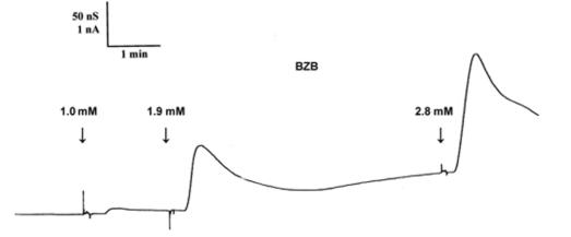
Figure 4. Recording of PC/n-decane membrane conductance measured at pH 7.35 after addition of BZB in increasing concentrations from 1.0 mM to 2.9 mM. doi:10.1371/journal.pone.0023187.q004
