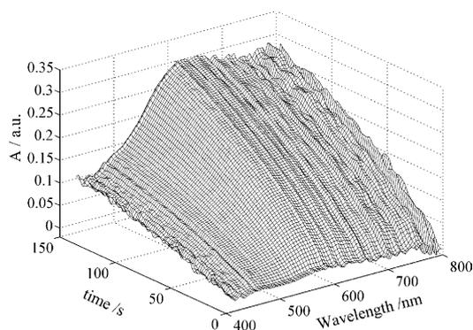
Fig. 5. 3D plot absorbance/time/wavelength in normal spectroelectrochemical arrangement for electropolymerisation of  $3 \times 10^{-3}$  M EDOT in 0.3 M LiClO<sub>4</sub> aqueous solution.  $E = +0.95$  V;  $t = 140$  s.
