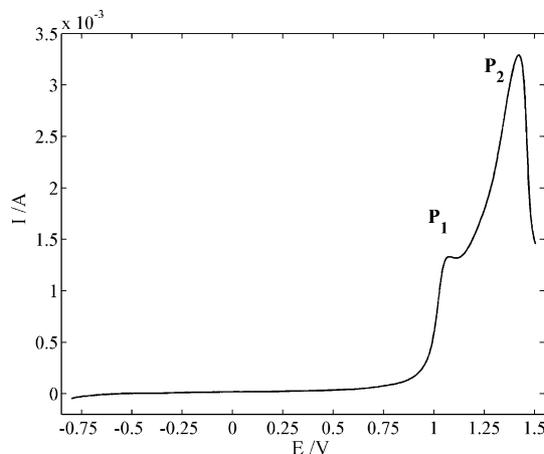
Fig. 2. Linear voltammogram of  $3 \times 10^{-3}$  M EDOT in 0.3 M LiClO<sub>4</sub> aqueous solution at  $0.05 \text{ V s}^{-1}$  using a gold working electrode.
