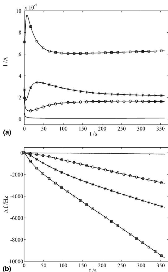
Fig. 3. (a) Chronoamperograms and (b) corresponding  $\Delta f$  vs.  $t$  plot in the electropolymerisation of  $3 \times 10^{-3}$  M EDOT in 0.3 M  $\text{LiClO}_4$  aqueous solution at (—) +0.75 V, (o) +0.80 V, (\*) +0.85 V and ( $\square$ ) +0.90 V.
