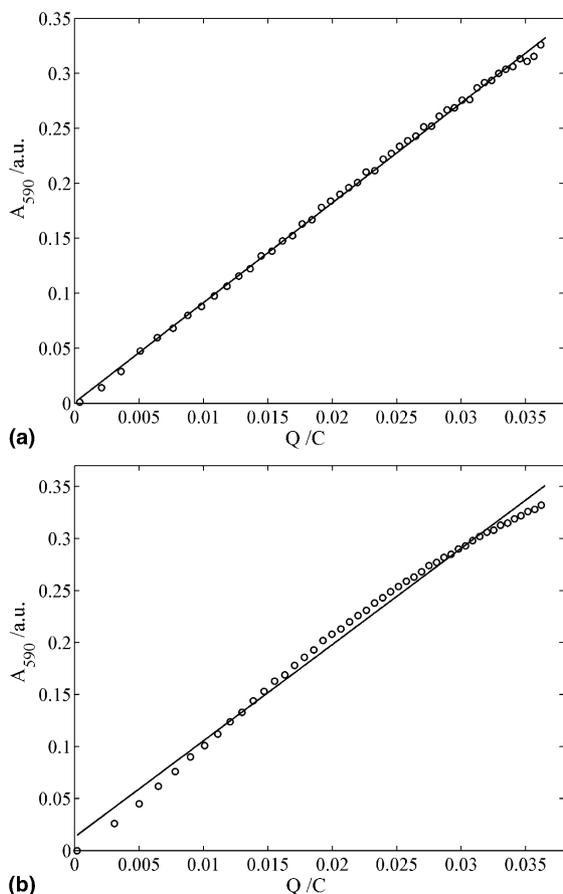
Fig. 7. Absorbance-charge relationships during electropolymerisation of  $3 \times 10^{-3}$  M EDOT in 0.3 M  $\text{LiClO}_4$  aqueous solution when the applied potential is (a) +0.95 V during 140 s or (b) +1.05 V during 120 s. Experimental data (o) and data fitted to linear models (—).  $\lambda = 590$  nm.
