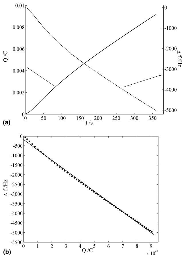
Fig. 4. (a)  $Q$  and  $\Delta f$  vs.  $t$  plots and (b)  $\Delta f$  vs.  $Q$  relationship during electropolymerisation of  $3 \times 10^{-3}$  M EDOT in 0.3 M  $\text{LiClO}_4$  aqueous solution at +0.85 V during 360 s.
