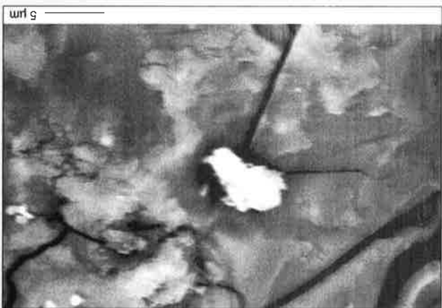
Figure 1 - SEM micrograph of glass doped with 10 wt% of \text{ZnO} after 2 weeks of soaking in SBF.
