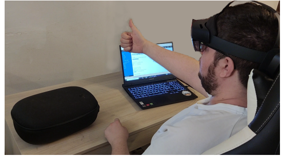
Fig. 1: Gesture acquisition: the subject hears vocal commands suggesting pre-defined sequences of non-significant movements and gestures.
