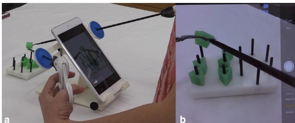
**Figure 2.** (a) Full assembled UCi Trainer with instruments and an iPad, (b) iPad view. (Color version available online.)
