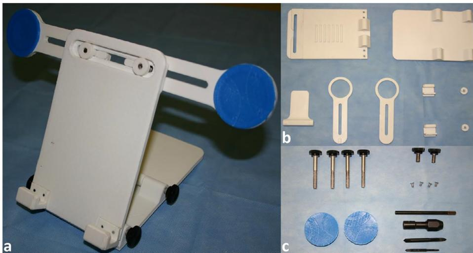
**Figure 1.** (a) Full assembled UCi Trainer, (b) 3D printed UCiT components, (c) Nonprinted UCiT components. (Color version available online.)
