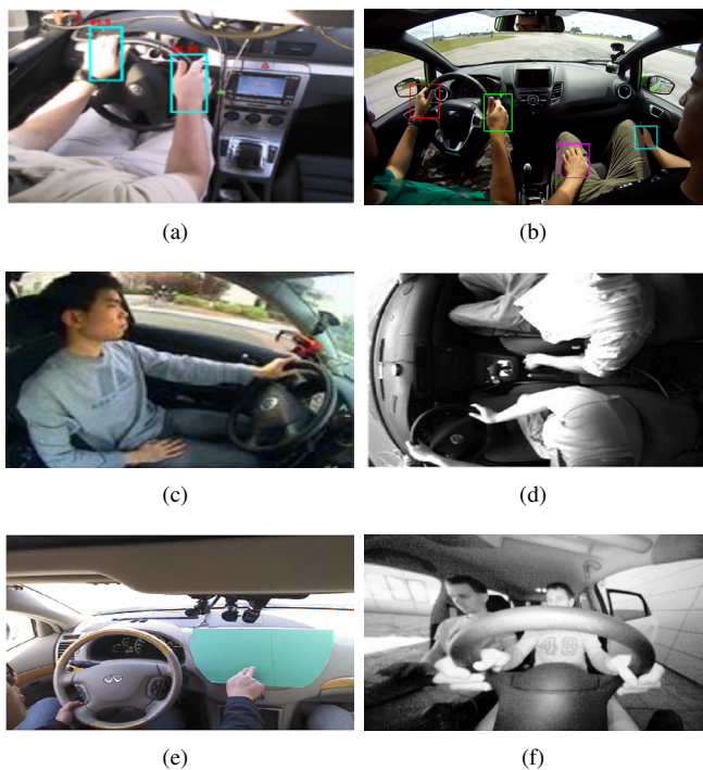
Fig. 1. Typical points of view for hand detection and tracking datasets in automotive. In particular, (a, b) are taken from [8], (c) [9], (d) [10], (e) [11] and (f) shows our innovative point of view. The fish-eye infrared camera is placed back to the steering wheel, very close to the hands.
