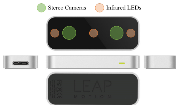
Fig. 2. Different views of the Leap Motion device. The position of stereo cameras and infrared LEDs are shown. The original image is taken from the official website [26].
