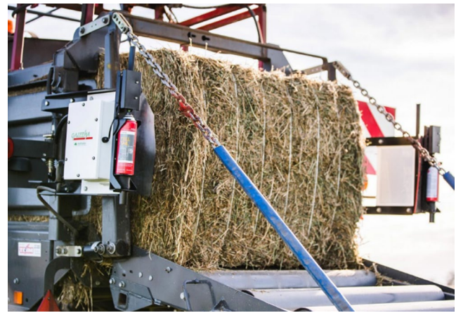
FIGURE 3 | Hay moisture meter for large square balers based on transmission of high frequency electromagnetic waves ( https://vomax.com.au ).
