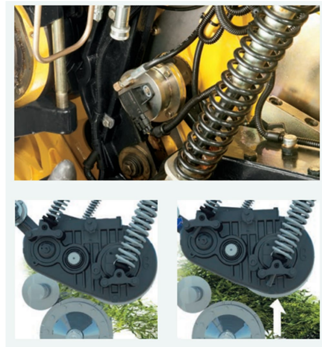
FIGURE 4 | Yield monitoring system based on continuously measuring of the opening of the feedrolls proposed by New Holland in his FR series forage harvesters. (New Holland 2024a, 2024b)
