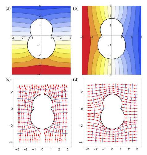
Figure 3. Temperature and heat flow fields for  $\beta_1 = \pi/3$ ,  $\beta_2 = -\pi/4$ , for the remote heat flux  $q_0$  along the axial (a and c) and transversal (b and d) directions.
