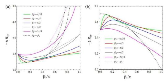
**Figure 5.** Normalized variations of the components of the resistivity contribution tensor of an equivalent insulating spheroid for some selected values of  $\beta_2$  varying  $\beta_1$ . Solid and dash-dotted curves are obtained for approximating spheroids with aspect ratios given by equations (48) and (49), respectively [AQ: 7].
