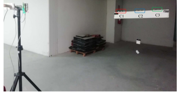
Fig. 9. Experimental setup developed for our acquisitions. The employed radar device is mounted on a wooden bar; the targets are small coins placed on a polystyrene plate.
