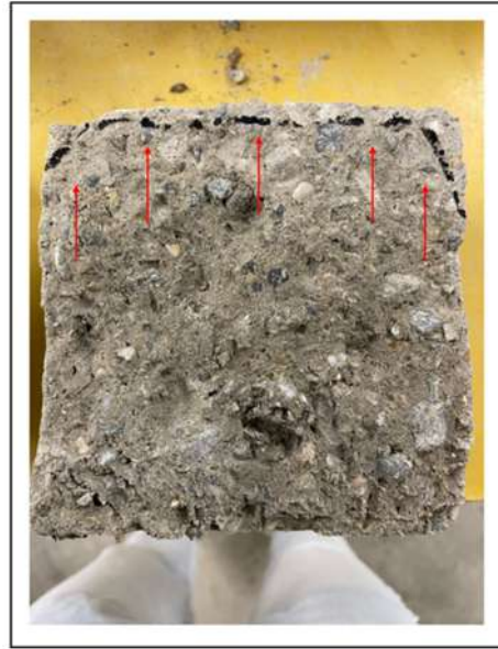
Fig. 6. Example of visible waterfront in SE1 after pressure exposure
