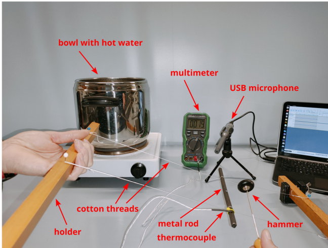
Fig. 2. Photo of the experimental setup. The bar (either the nitinol or the iron bar) is tied to two rigid holders with cotton threads passing at the nodal planes of the bar. A thermocouple is fixed to the bar and the temperature is read by a multimeter. Using the holders, the bar is first immersed in a bowl containing water at a fixed temperature. Then, it is quickly extracted from water and held suspended with the holders. As the bar gradually cools, the operator may repeatedly take note of (or read aloud for recording) the temperature from the multimeter and gently hit the bar with a rubber hammer. The sound is recorded through a microphone connected to a computer to be analyzed.
