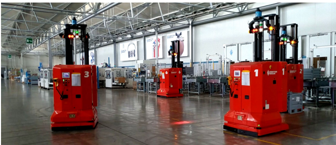
Fig. 11. A photo taken during the experiments conducted in the automated factory. The 4 AGVs are coordinating in a load and unload cargo area.
