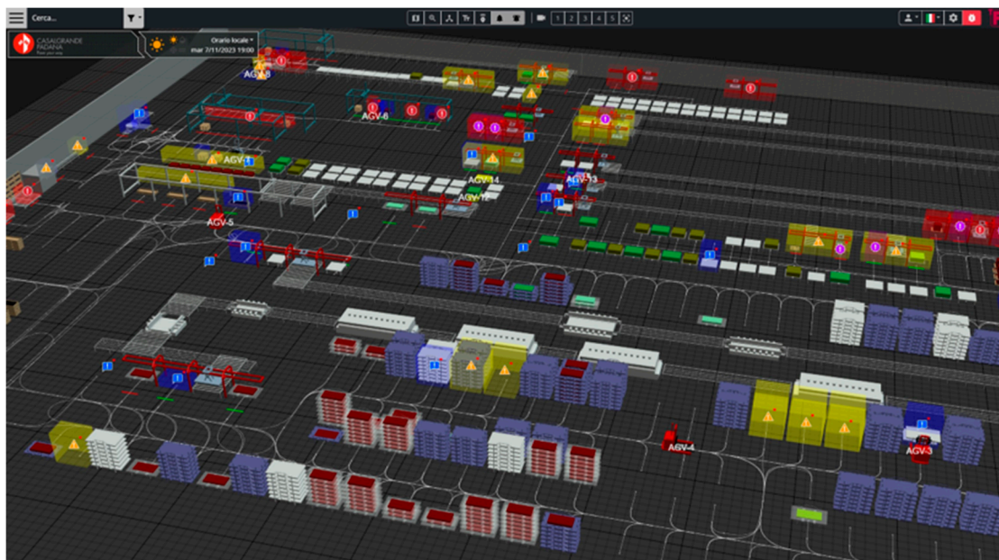
Figure 14. Graphical 3D DT of the pilot production plant. The piles of product being stored, the trajectories of the AGVs, as well as the identifiers of the storage buffers are visible in the layout.
