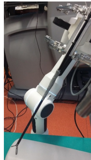
(b) three strain gauges applied on the SARAS laparoscopic tool after being covered with a protective material.
