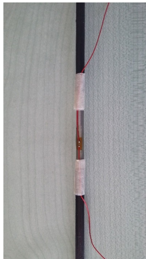
(a) a single strain gauge applied on the laparoscopic tool before being covered with a protective material.
