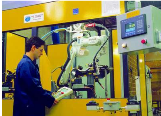
Figure 9: Lead-through programming by teach pendant.
