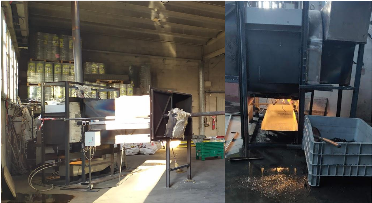
Figure 15 Melting furnace and slag outlet segment from the melting furnace and water-cooling tank
