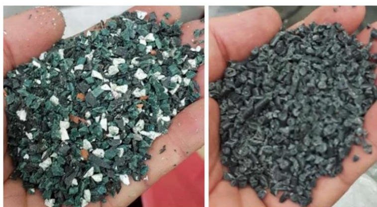
Figure 35 Comparison of polyolefins before (left) and after (right) homogenization treatment
