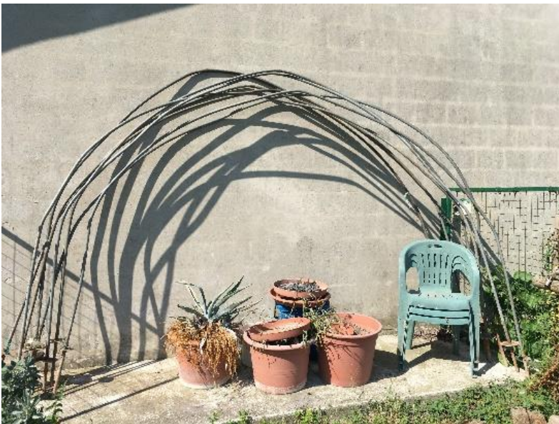
Figure 6: metal tubes used in the building of the greenhouse
