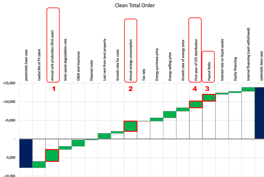
Fig. 10. Breakdown of ΔNPV e from the pessimistic base scenario to the optimistic base scenario.
