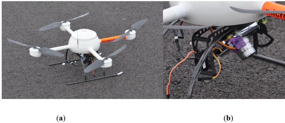
Figure 6. (a) Microdrones md4-200. (b) Detail of digital camera Pentax Optio A40 and gimbal on board.
