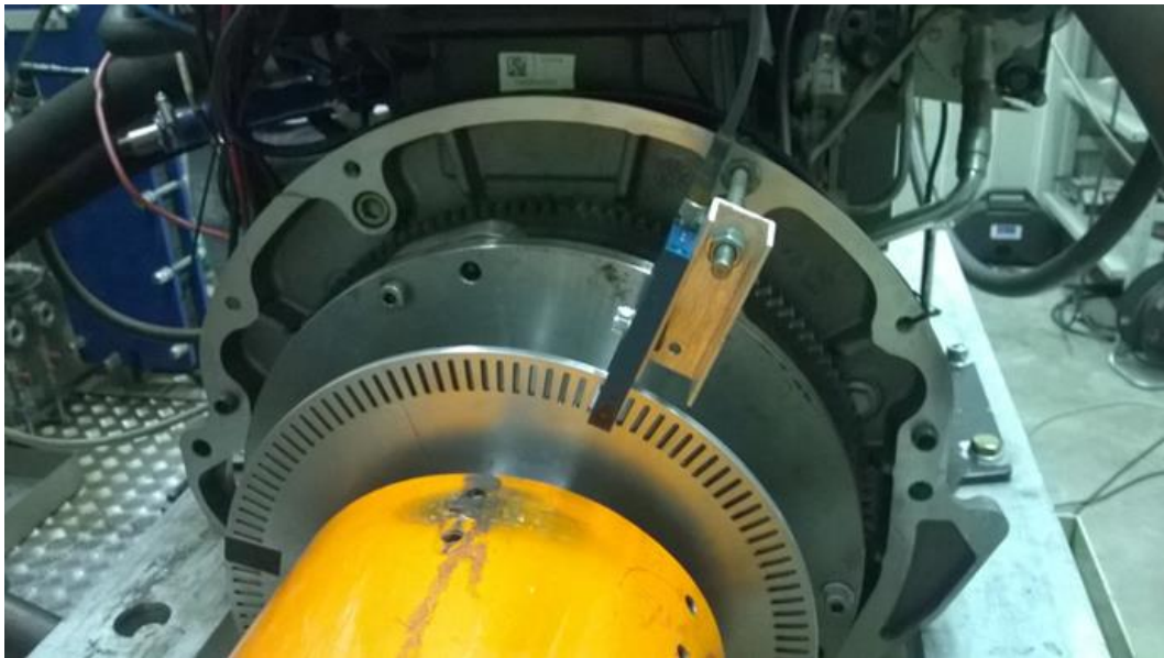
Figure 4.10 - Optical encoder and sound wheel located on the drive shaft exit
