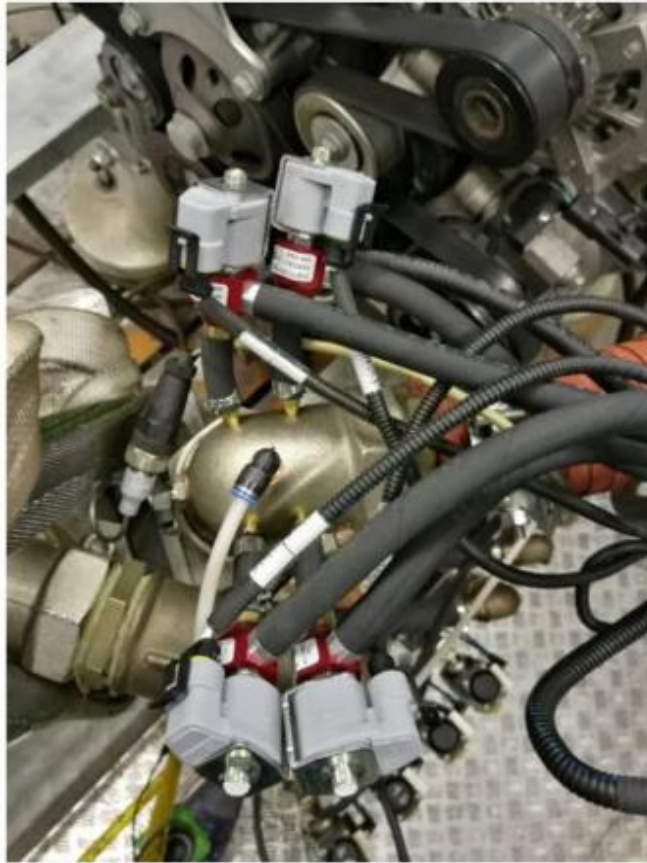
Figure 4.15 - Methane injection system installed after the intercooler
