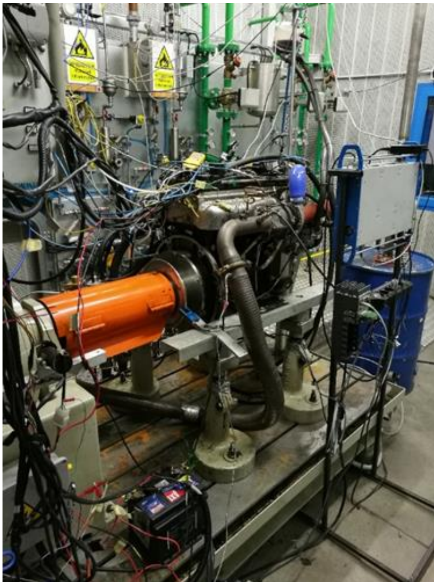
Figure 4.20 - Engine installed on the Unimore test bench
