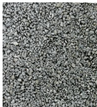
Sample B: Asphalt Shingle treated with TiO 2 and hydrophobic treatment
