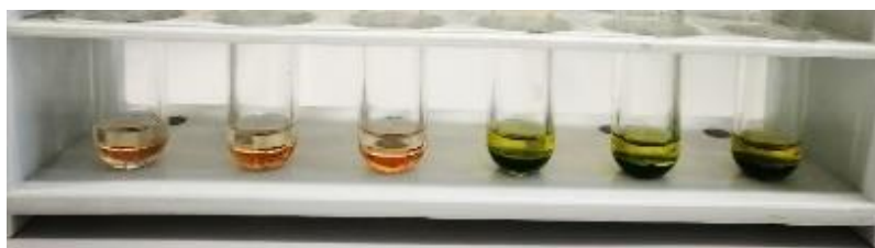
Figure 55: Two-phases fatty acids extractions: polar phase is the upper layer and the lower phase contains fatty acids. Two algal species FA extraction are shown ( K. flaccidum on the left and E. mirabilis on the right).
