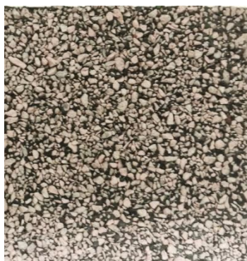
Sample A: Asphalt Shingle treated with CuO, ZnO and TiO 2
