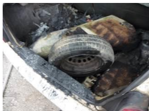
Fig. 6 Photos of the interior of the central car used in test C1SPK: a) before and b) after testing
