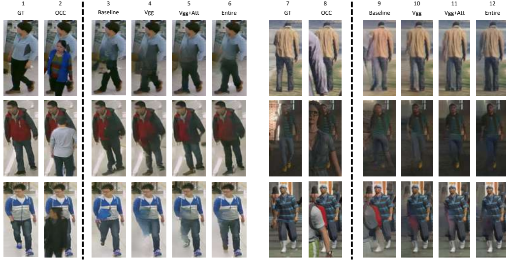
Fig. 9. Qualitative results based on the ablation study on RAP dataset (leftmost) and AiC dataset (rightmost). GT columns indicate ground truth images while in the OCC columns are presented the input occluded images. Columns 3 and 9 indicate the outputs of our baseline. Columns 4 and 10 represents results of the VGG loss. On 5 and 11 we have results of experiments using all the 3 losses combined: adversarial loss, VGG loss, and attribute loss. Finally, columns 6 and 12 show results where attributes are injected as input to the network. The Figure is taken from “Can Adversarial Networks Hallucinate Occluded People With a Plausible Aspect?” [17]
