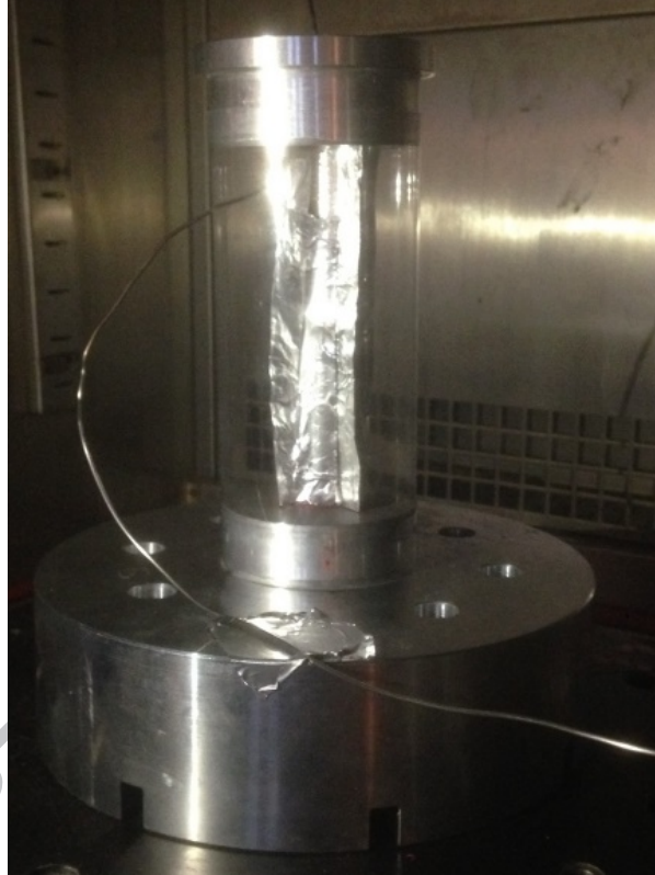
Figure 9 – Set-up for axial forcing load tests with thermic gradient
