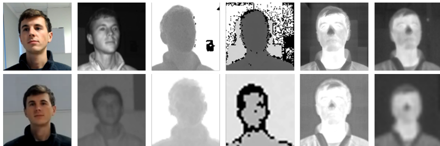
Figure 3.1: Samples from the MultiSFace dataset. In the first row, the subject is near the sensors (1 m distance) while in the second row the subject is far from the sensors (2.5 m distance). Starting from the left: RGB and infrared images, high- and low-resolution depth maps, and high- and low-resolution thermal images.
