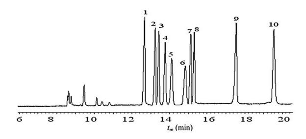
Figure 4. CE-C4D separation of a mixture of saccharides. Optimized conditions are: BGE 75 mM NaOH pH 12.81, capillary i.d. 5  $\mu$ m, total length 32.6 cm, length to the detector 18.3 cm. Hydrodynamic injection at a pressure of 50 mbar for 80 s. Voltage, +15 kV, current 1.6  $\mu$ A. Sample concentration, 100 mg/L in 50% v/v acetonitrile. Peak identification: 1, sucrose; 2, lactose; 3, galactose; 4, glucose; 5, mannose; 6, fructose and 7, ribose. Reprinted with permission from Reference [39].
