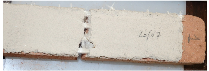
Fig. 7. Typical telescopic failure mode for brick bending in the G-UC specimen group.
