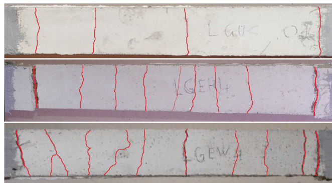
Fig. 15. Near failure crack pattern in G-UC (top), G-ER (middle) and G-EW (bottom) specimens.
