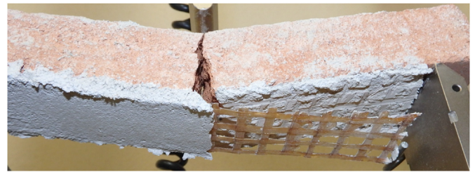
Fig. 8. Typical delamination failure mode for brick bending in the G-ER and G-EW groups.
