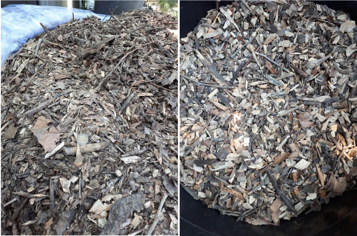
Figure 4: Green waste sample before and after the sieving and drying processes
