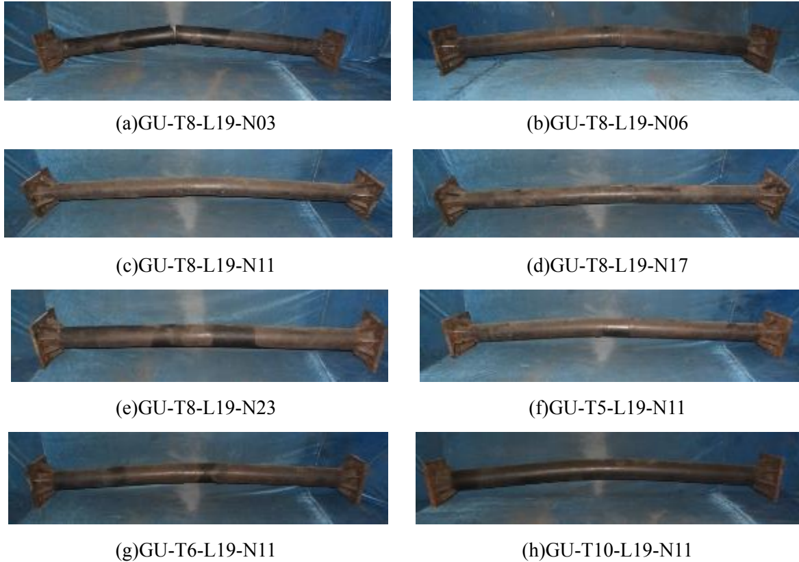
Fig. 2-11 Integral bending failure diagram of UCFST columns
