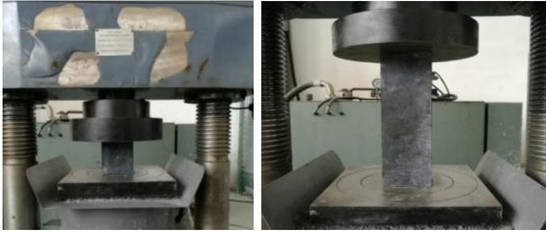
(a) UHPC cube specimen (b) UHPC prism specimen
