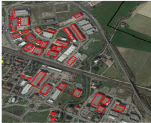
Figure 17-7: Vector mapping of AC sheeting superimposed on the Cadastral Map (AeroDron AsbestosFree)
