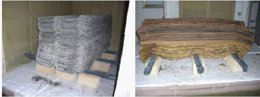
Figure 17-22: Left: package of asbestos cement sheets before thermal treatment; right: package of asbestos cement sheets after thermal treatment.
