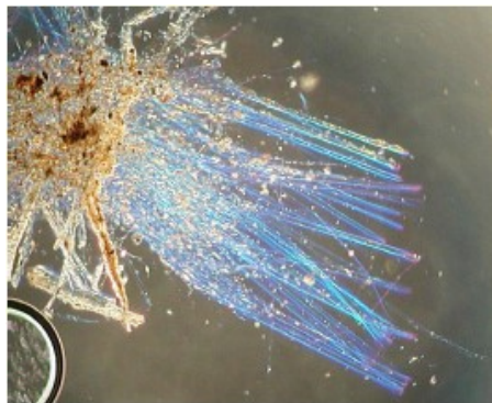
Figure 12-6: MOCF of fibers of chrysotile seen by the chromatic dispersion method
