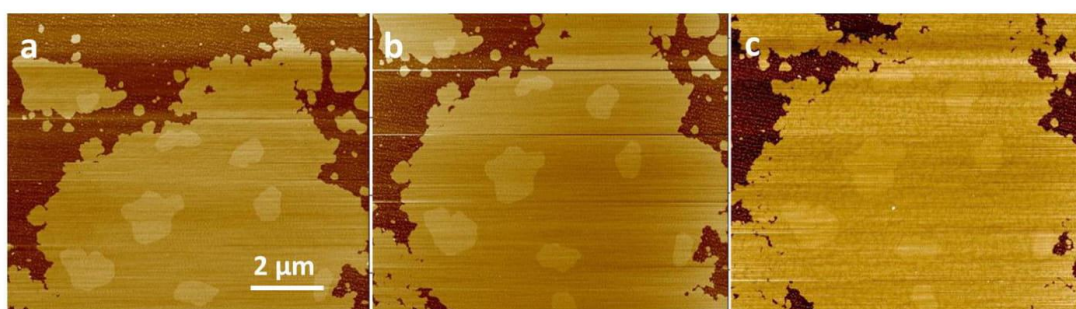
Figure S3: a) POPE/POPG 3:1 SLB imaged at 20°C; b) the same area of a) is imaged immediately after DAP has been added to the imaging chamber in order to have 3 \mu\text{M} DAP concentration: we observe an immediate increase of the lipid bilayer area; c) the same area of a) with 3 \mu\text{M} DAP concentration 10 minutes after the lipopeptide has been added. The bilayer shows a strong reorganization of its phase state, with higher domains appearing in the previously completely fluid regions.
