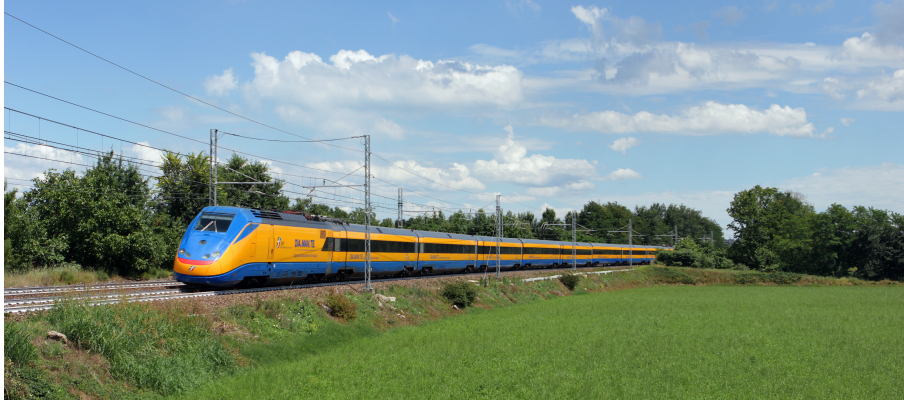
Figure 3.1: ETR.500 Y 2 “Dia.man.te”, high speed (300 km/h) visual inspection EMU (for track and catenary) of Rete Ferroviaria Italiana (RFI), Italian railway’s infrastructure manager. Courtesy of © Stefano Paolini.
