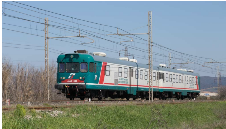
Figure 3.3: “us1-Galileo,” conventional ultrasonic measure train of Rete Ferroviaria Italiana (RFI), Italian railways infrastructure manager. Courtesy of © Benedetto Sabatini.
