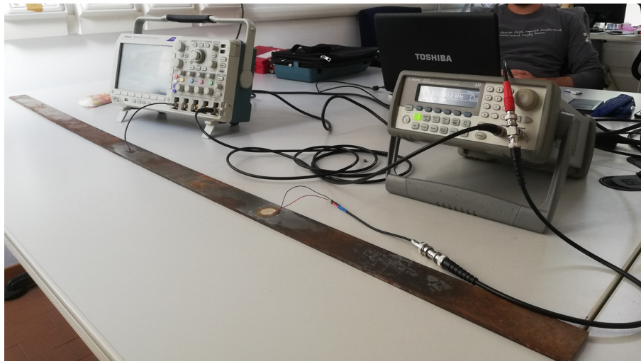
Figure 12.6: Picture of the bar and of the instrumentation used in our qualitative experiments.
