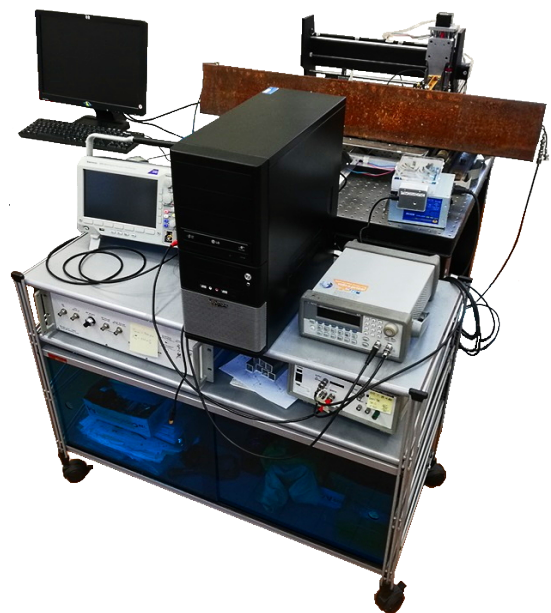
Figure 12.25: Measurement set-up for the experimental observation of the dispersion curves of a rail.
