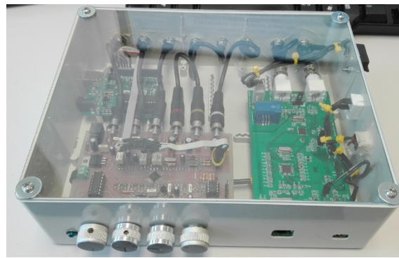
Figure 18.4: TCCSA track circuit signal demodulator.
