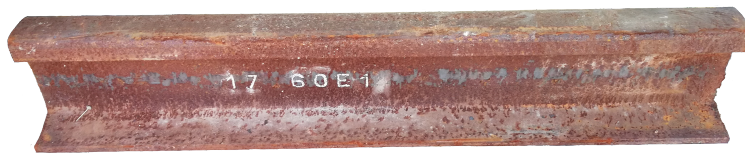
Figure 12.27: Section of rail used as a waveguide.
