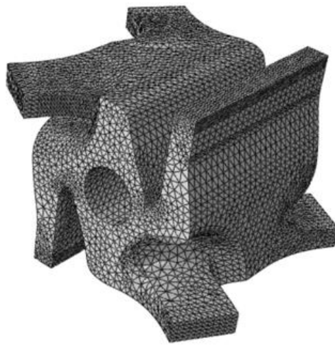
Figure 49 Rotating cube element with FE mesh.
