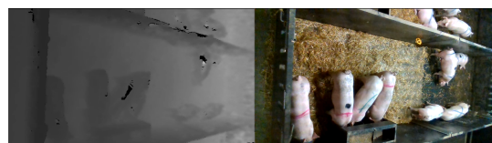
Figure 1: An example of depth and RGB data for the same frame. The depth data has several artifacts. One of the pigs in front of the feeder has a wide (black) spot with value zero, while one in the rear has both zero and out of distribution (white patch) areas.
