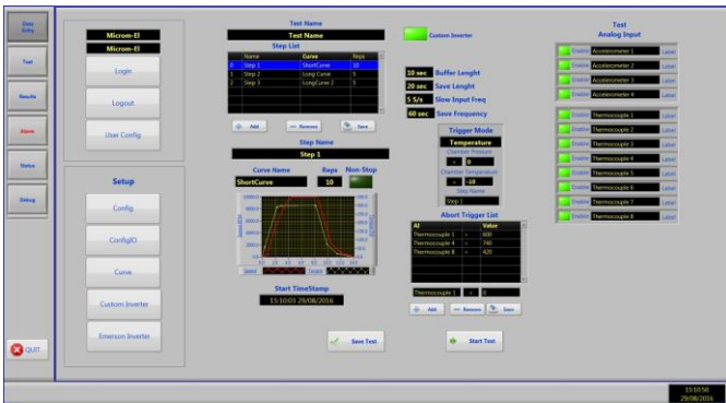
Fig. 14 Control interface data entry panel.
