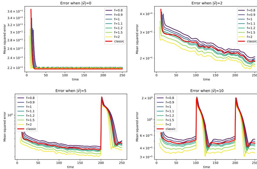
**Fig. 2.** Root mean squared error for diverse  $v$ . When the network is entirely static (top left), after a short stabilization time the network converges to a very low error. Errors are lower with higher  $f$  values. The performance with  $f = 1$  is equivalent with the performance of the baseline. When  $\|v\| \geq 5$ , there is enough time for the mobile device to leave the system and for a new one to join, creating a spike in error and requiring a re-stabilization.
