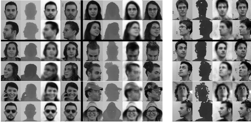
Figure 4.8: Test (a) and train (c) images on Pandora dataset, test (b) and train (d) images on Biwi dataset. For each block, gray-level images and then the corresponding depth faces are depicted in the first columns; face images taken from the method described by Borghi et al. are reported in the third column; finally, the output of the Face-from-Depth network proposed in this work is depicted in the last column.
