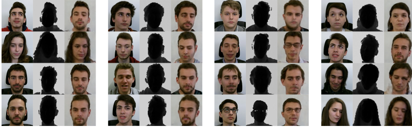
Figure 4.12: Best results on the MotorMark dataset. For each triplets of images: (Leftmost) the original image; (Middle) the input depth map; (Rightmost) the Generated face image.
