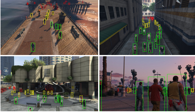
Figure 3.22: Examples from the JTA dataset exhibiting its variety in viewpoints, number of people and scenarios. Ground truth bounding boxes are superimposed to the original images. Green color is used for people having a distance from the camera between 0 and 20 meters, yellow for people between 20 and 40 meters and red for people between 40 and 100 meters.
