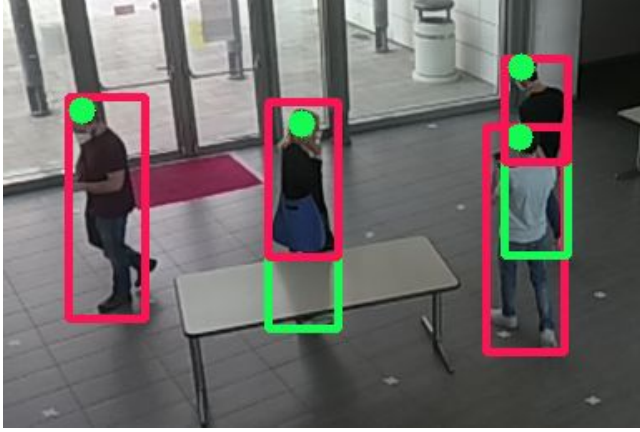
Figure 3.20: Examples of CenterNet bounding boxes (pink), refined bounding boxes and head localization (green).
