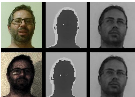
Figure 4.2: Example of reliability of the FfD network on depth images. Two consecutive frames have been selected from a sequence with an abrupt illumination change (from light to dark). In the first column the auto equalized RGB, then the corresponding depth maps and finally the FfD reconstruction output.
