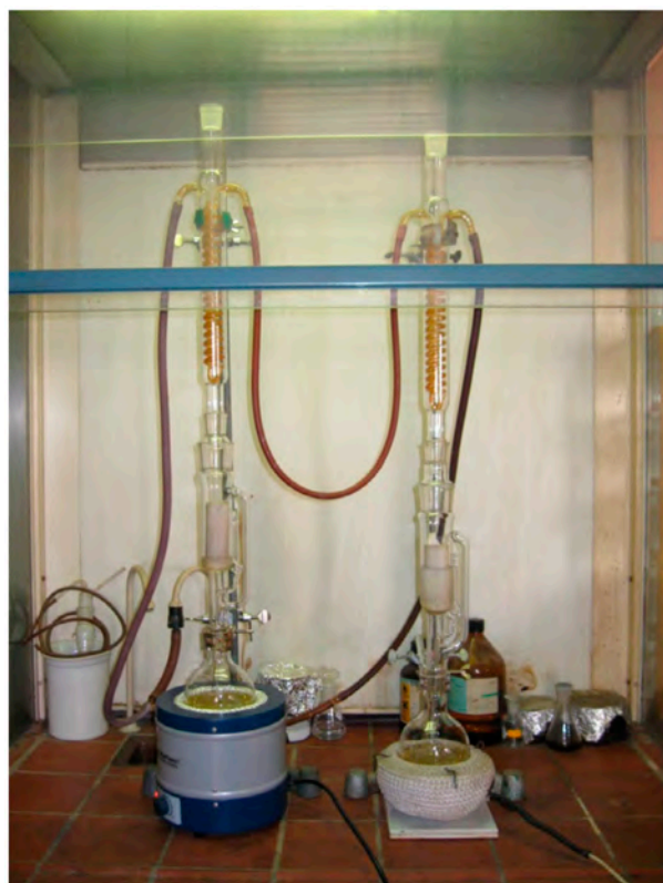
Figure 14. Determining the wax content of propolis by Soxhlet extraction.
