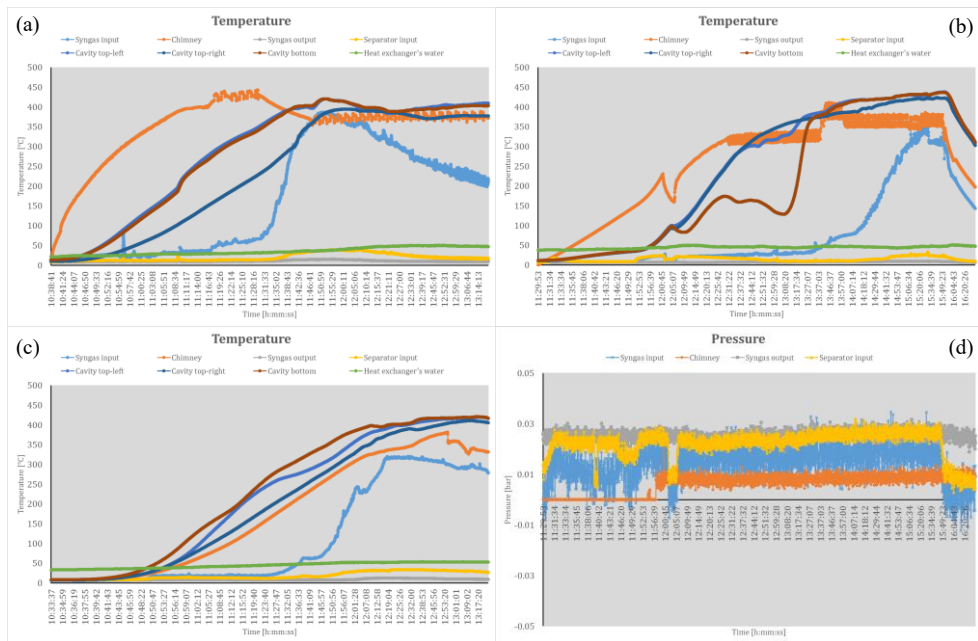
Fig. 4. (a) Waste tires pyrolysis temperatures graph, (b) Polyethylene bags pyrolysis temperatures graph, (c) Rubber fabric and vulcanized pipes waste pyrolysis temperatures graph, (d) Polyethylene bags pyrolysis pressures graph
