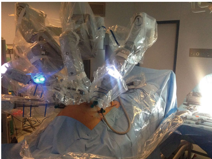
FIGURE 56.7 The robotic arm system is docked to the patient with a “side docking” approach
