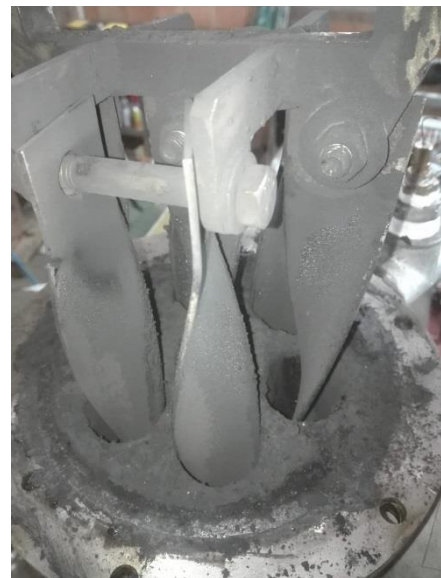
Figure 58. Soot deposition on the top of the heat exchanger: rack of twisted tapes after the tests.
