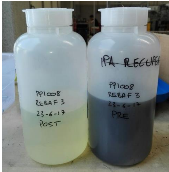
Figure 38. IPA collected downstream (left) and upstream (right) the filtration stage.
