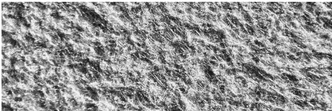
Figure 62. Texture of the filtrating mesh of a PE bag.
