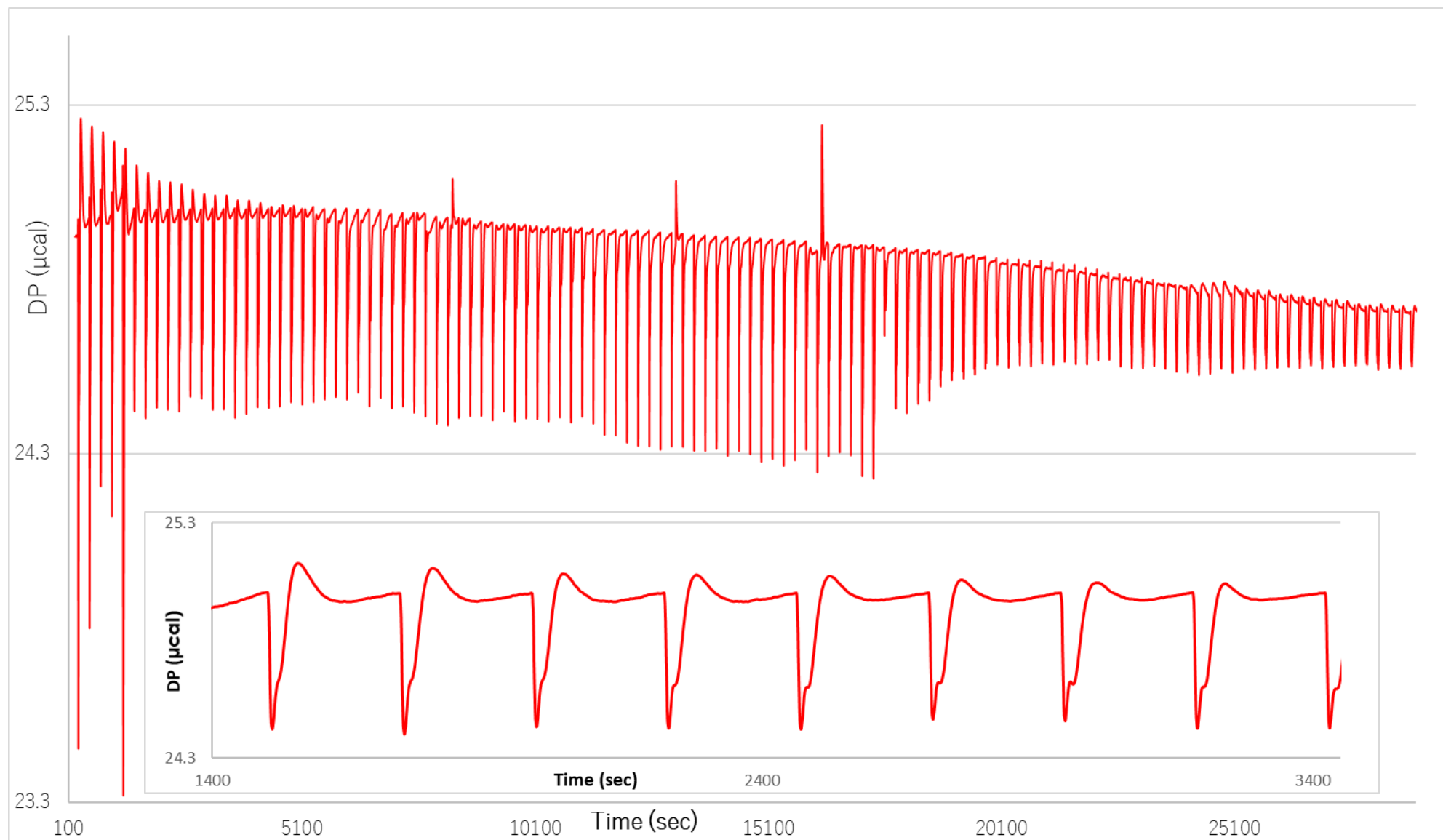
Graph 15: ITC data result from the subtraction of control titration - no protein - from the hTSwt titration with dUMP.
