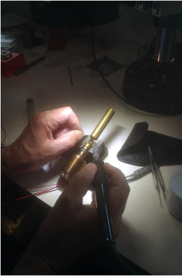
Figure 5.11 (a and b): Furnace containing the threaded Teflon lined capsule for the large-volume HP experiment.
