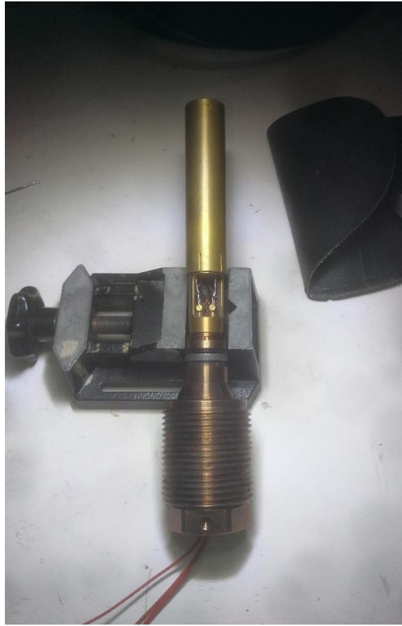
Figure 5.11 (a and b): Furnace containing the threaded Teflon lined capsule for the large-volume HP experiment.
