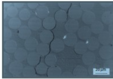
Figure 3.1 . Debonds in a fiber- reinforced composite. From Compos Sci Technol, Vol 59, E.K. Gamsted and B.A. Sjorgren, Micromechanisms in tension-compression fatigue of composite laminates containing transverse plies, pp. 167-78, copyright Elsevier (1999).
