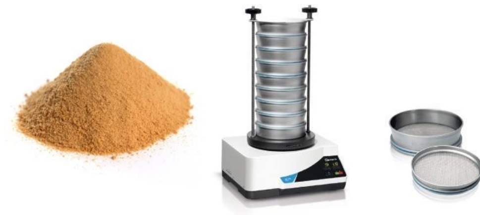
Figure 7.2: Separation of powder with the sieving equipment into its granulometric fractions
