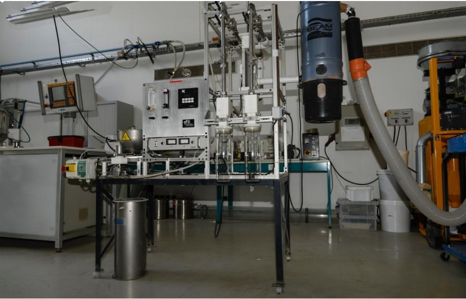
Figure 46: Electrostatic separation pilot plant
