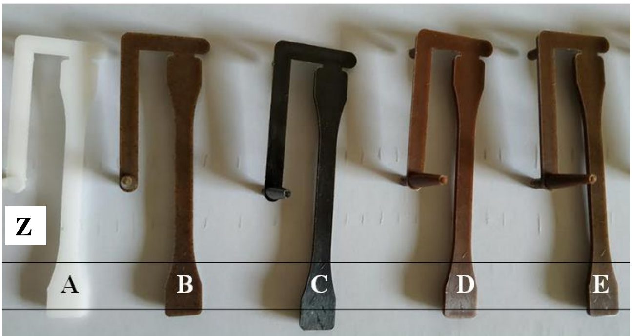
Figure 8.11: (Y) Extruded bio-composite materials wrapped in reels. (Z) Bio-composites obtained from grape stalk powders. From left to right: (A) PBS specimen, (B) PBS 10 GS specimen, (C) PBS 10 GS acetylated specimen, (D) PBS 10 GS specimens, and (E) PBS 10 GS silylated in situ.
