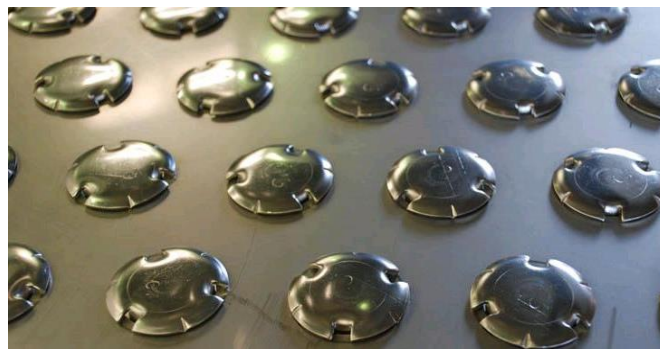
Figure 49: Valve plates for the distillation column
