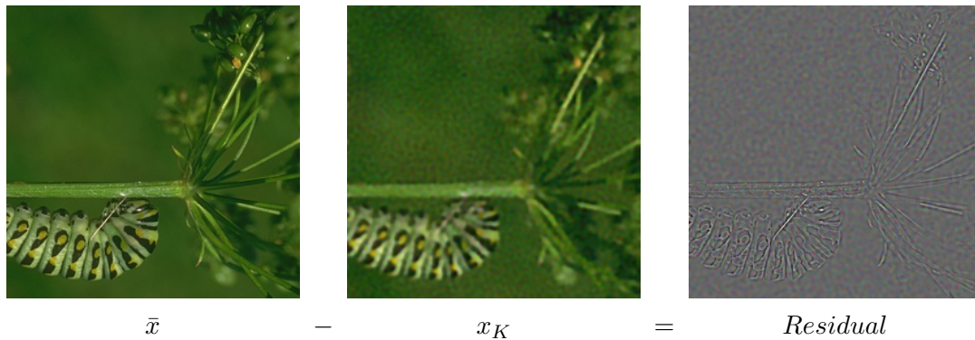
Figure 4.4: Remaining artifacts given by the difference between a ground-truth image and x_K obtained with the network trained for the experimental GaussianB configuration.
