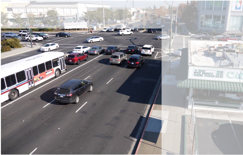
Figure 4.4: Example of considered Region of Interest (ROI) for location 4 of NVIDIA AI city challenge. It can be appreciated how the farthest vehicles are ignored, thus trading off the detector recall for an improved precision. Ignored detections usually correspond to the farthest vehicles, which would be anyway very hard to track correctly. Since in the successive phase tracklets are used as ground truth annotations for the challenge videos we choose to privilege the precision w.r.t. the recall of the tracker.
