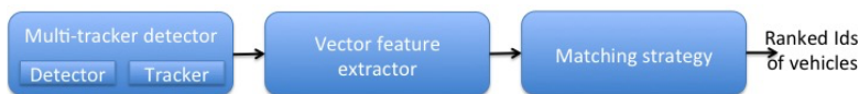
Figure 4.2: Our re-identification pipeline that is composed of three modules. The first phase is vehicle detection and tracking. Detections are either assigned to an existing tracklet or used to initialize a new tracker. Tracklets are exploited to automatically annotate the videos and train a triplet network for vehicle re-identification. The output vector of the triplet network is used as feature vector to represent each detected vehicle. Eventually, these feature vectors are compared between different probes and the gallery to generate a ranking. We refer the reader to Section 4.1.1 for further details.
