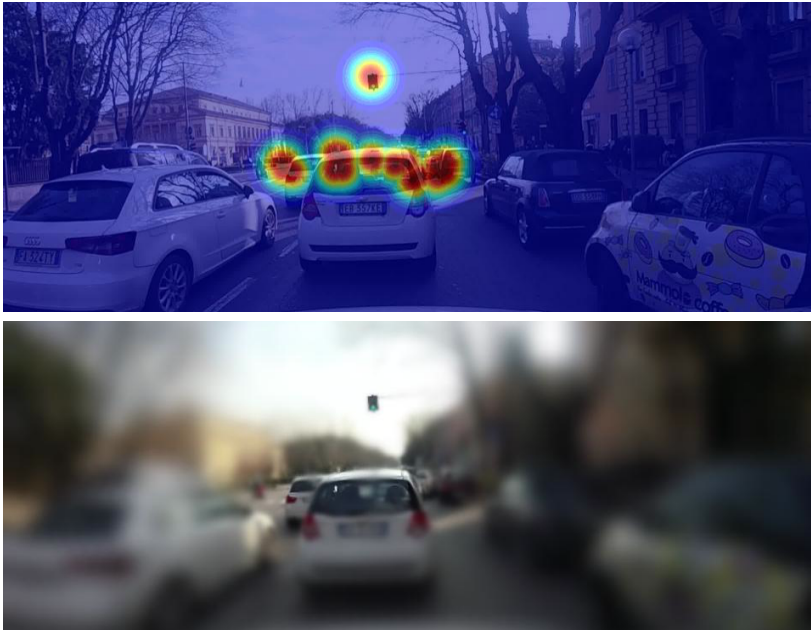
Figure 3.25: The figure depicts a videoclip frame that underwent the foveation process. The attentional map (above) is employed to blur the frame in a way that approximates the foveal vision of the driver[137]. In the foveated frame (below), it can be appreciated how the ratio of high-level information smoothly degrades getting farther from fixation points.
