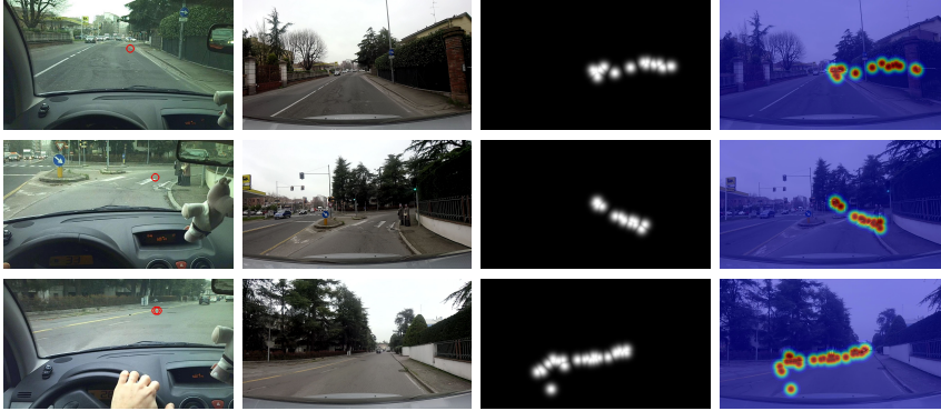
Figure 3.16: Examples taken from a random sequence of DR(eye)VE . From left to right: frames from the eye tracking glasses with gaze data, from the roof-mounted camera, temporal aggregated fixation maps (as defined in Sec. 3.1.2) and overlays between frames and fixation maps.
