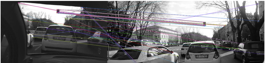
Figure 3.3: Registration between the egocentric and roof-mounted camera views by means of SIFT descriptor matching.
