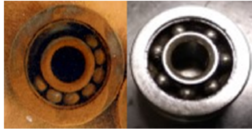
Figure 4.11: From the left to the right: (1) Bearing during water treatment (2) Rusty bearing after the removal of the rust.
