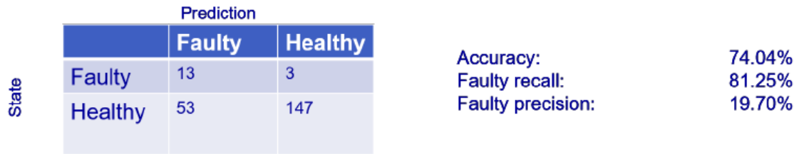
Figure 4.48: Confusion Matrix of "OR" prediction between Random Forest Binary Classifier and SVM Binary Classifier.
