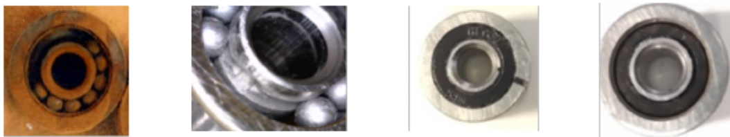
Figure 4.10: Damaged bearing images, from the left to the right: (1) Rusty bearing, (2) Bearing with an inner ring damage, (3) Bearing with an outer ring damage, (4) Blocked bearing.
