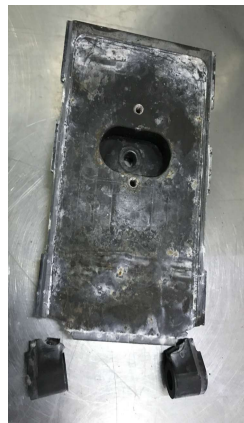
Figure 76: Volume Box broken on in operation
