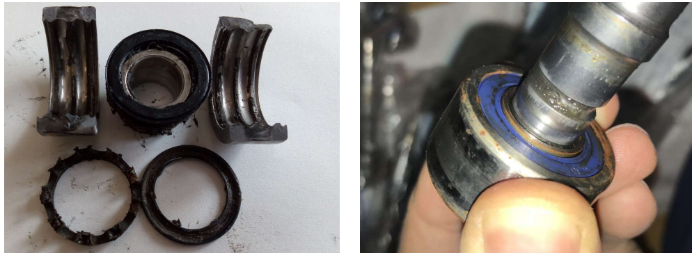
Figure 124: Test Rig damaged bearing
