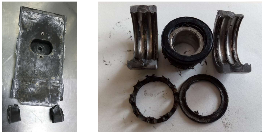
Figure 128: Failures: Volume Flap (left) and Ball Bearing (right)
