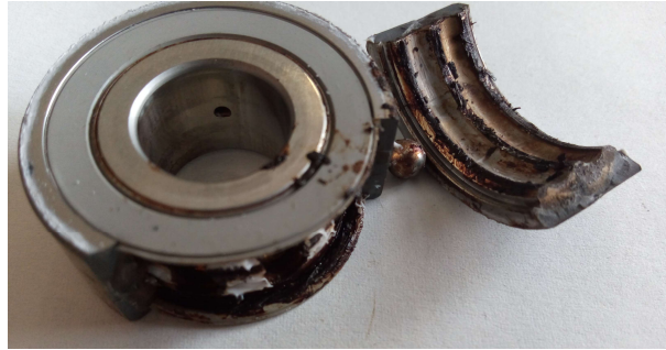
Figure 123: Test Rig damaged bearing
