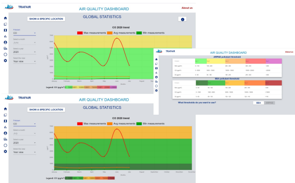
Fig. 6. Two year views for CO in 2020: the bottom uses ARPAE scale and the top EEA scale. The figure shows also the setting view where scales can be modified.
